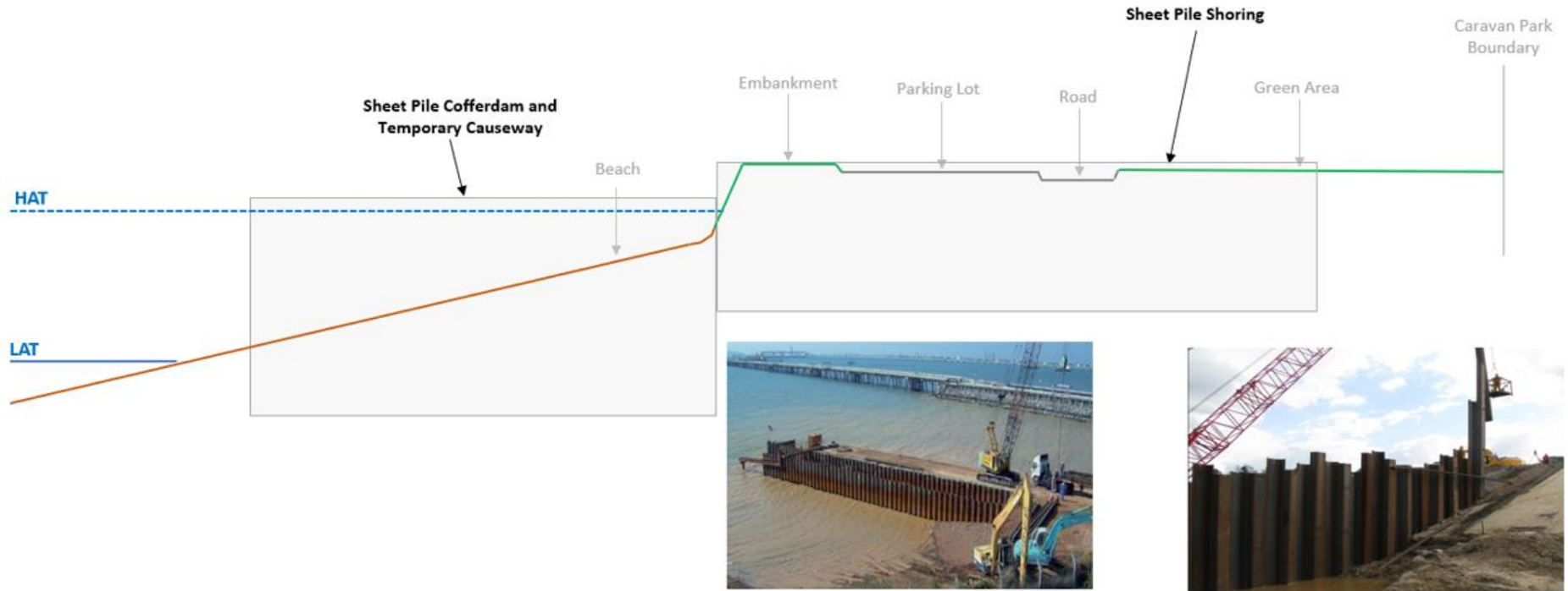
Figure 2.6 Temporary Works – Cofferdam and Causeway Construction
